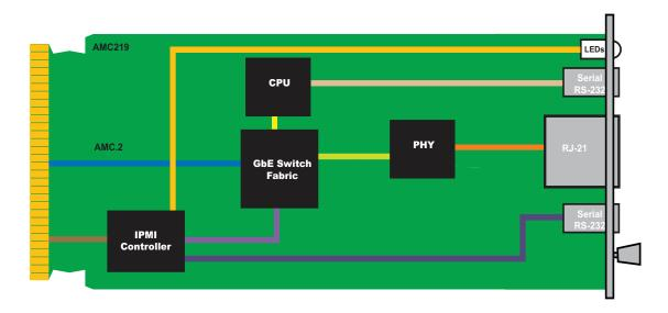
FIGURE 1. AMC219 Functional Block Diagram
